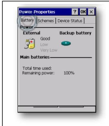
9.2.3 Selecting **Battery** displays the status of the main and backup batteries and the percentage of remaining power.
