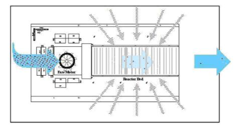
Contaminated air is drawn into the AiroCide system by the fan. It passes over the reactor bed where it is immobilized on the TiO2 catalyst and treated with UV-light until it is completely broken down to gaseous products. The combination of TiO2 catalyst and UV-light has been shown to destroy hydrocarbon bonds in allergens, airborne organisms and VOC's.
