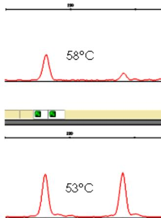
Example: Reduced efficiency of amplification of the longer allele. Repeating PCR amplification with an annealing temperature 5°C lower may help to confirm that the unusual result is due to a mutation in the STR primer binding site.
