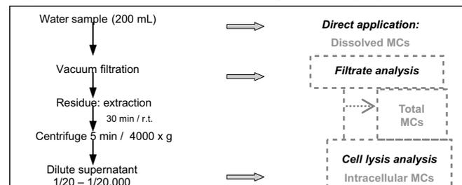
Scheme procedure for water samples from reservoirs, rivers, etc.
